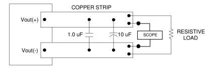
Note: Use a  $1.0\mu F$  X7R ceramic capacitor and a  $10\mu F$  @ 25V tantalum capacitor. Scope measurement should be made using a BNC socket. Position the load 3 in. [76mm] from module.
