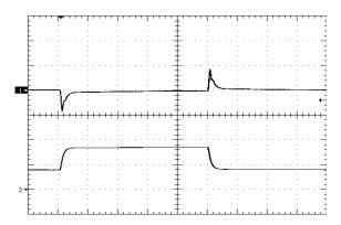
Figure 9. Load Transient Response di/dt=0.1A/uS, 25% - 50% - 25% of full load, time scale: 200uS/div Ch1=100mV/div, Ch2=2A/div
