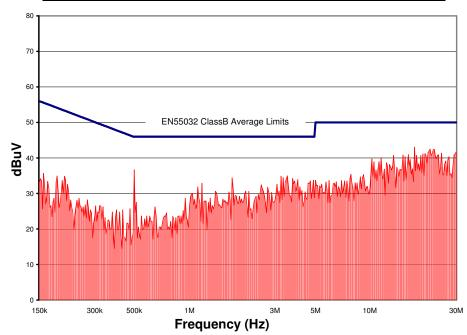
Figure 16. CPT7B24 Conducted Emissions using above specified input filter.
