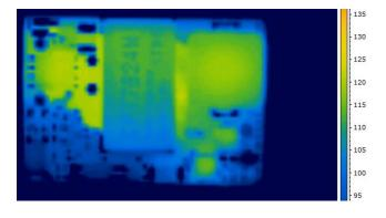
Figure 4. Thermal Image of CPT7B24 7A output, 45C Ambient, 200LFM, Vin = 24V, airflow from pin 3 to pin 1, T<sub>max</sub> = 123 °C
