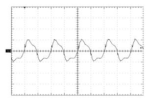
Figure 5. Output Voltage Ripple (20mV/div), time scale – 1uS/div. Vin=Vin\_nom, full resistive Cout=1uF ceramic + 10uF Tantalum (see Fig 12)
