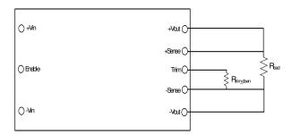
Figure 14. Trim DOWN circuit configuration
