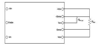
Figure 13. Trim UP circuit configuration
