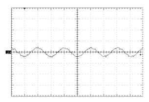
Figure 6. Input Reflected Ripple Current (10 mA/div) time scale - 1uS/div. Vin=Vin\_nom, full resistive (see Fig 11)
