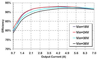
Figure 1. Efficiency vs Output Current, 300lfm airflow, 25  $^{\circ}\text{C}$  ambient.
