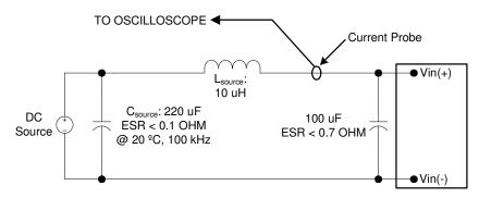
Note: Measure input reflected-ripple current with a simulated source inductance (Ltest) of 10 uH. Capacitor C<sub>S</sub> offsets possible source impedance.
