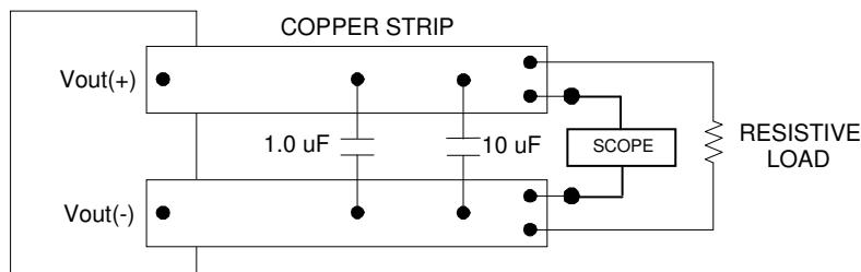
Note: Use a 1 $\mu$ F X7R ceramic capacitor and a 10 $\mu$ F X7R capacitor. Scope measurement should be made using a BNC socket. Position the load 3 in. [76mm] from module.
