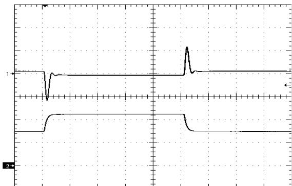
Figure 9. Load Transient Response
