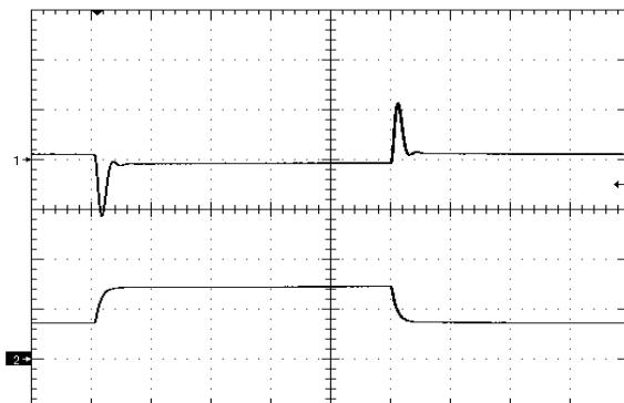
Figure 10. Load Transient Response (100mV/div), di/dt=0.1A/uS, 25% - 50% - 25% of full load, time scale: 200uS/div Ch1=100mV/div, Ch2=2A/div
