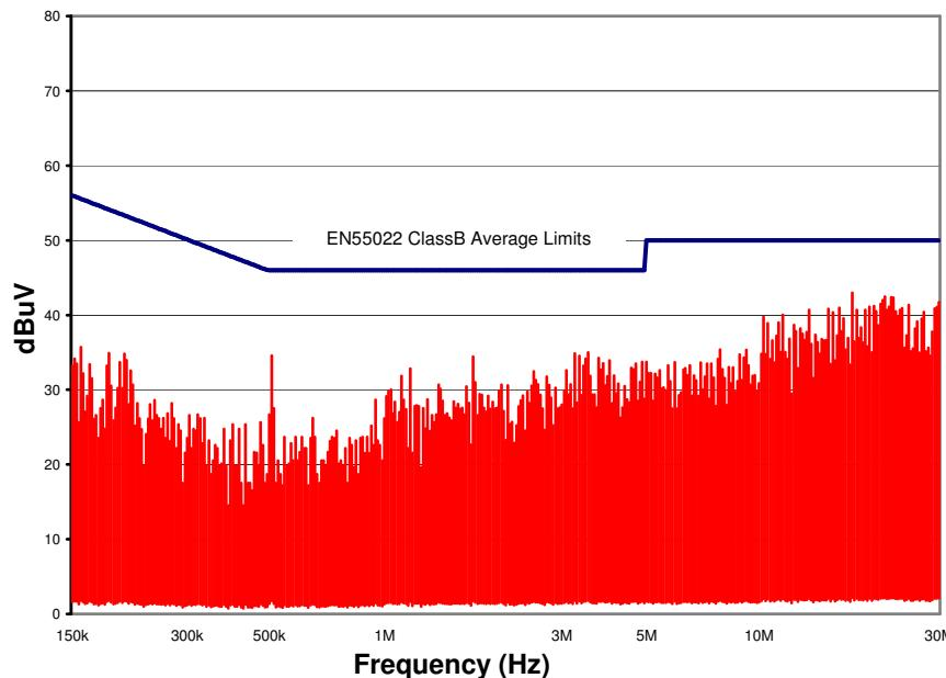
Figure 16. CPT6A48 Conducted Emissions using above specified input filter.
