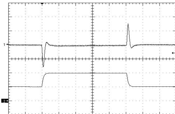
Figure 11. Load Transient Response (100mV/div), di/dt=0.1A/uS, 50% - 25% - 50% of full load, time scale: 200uS/div.
