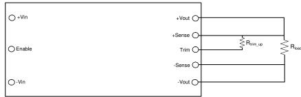
Figure 15. Trim UP circuit configuration
