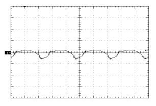
Figure 7. Output Voltage Ripple (50mV/div), time scale – 1uS/div. Vin=Vin\_nom, full resistive
