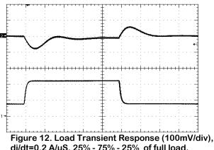
di/dt=0.2 A/uS, 25% - 75% - 25% of full load, 2000uF low ESR Oscon, time scale: 200uS/div
