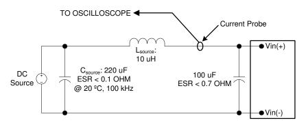
Note: Measure input reflected-ripple current with a simulated source inductance (Ltest) of 10 uH. Capacitor  $C_8$  offsets possible source impedance.
