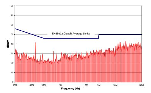
Figure 18. CPE6B18 Conducted Emissions using above specified input filter, Vin = 24V, Full Resistive Load
