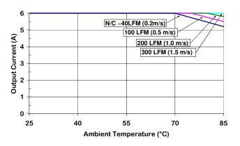
Figure 5. Output Current Derating vs Ambient Temperature & Airflow (air flowing from pin 3 to pin 1, <u>with</u> baseplate, Vin = 12-24 V.)
