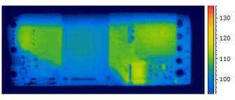
Figure 6. Thermal Image of CPE6B18 (6A output, 70C Ambient, 200Ifm airflow, Vin = 24V, airflow from pin 3 to pin 1, T<sub>max</sub> = 116 ℃)
