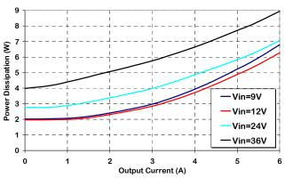
Figure 2. Power Dissipation vs. Load Current, 300lfm airflow, 25 ℃ ambient.
