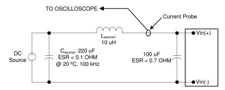
Note: Measure input reflected-ripple current with a simulated source inductance (Ltest) of 10 uH.
