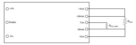
Figure 14. Trim DOWN circuit configuration
