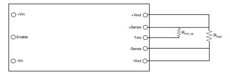
Figure 13. Trim UP circuit configuration
