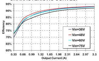
Figure 1. Efficiency vs Output Current, 300lfm airflow, 25 ℃ ambient.
