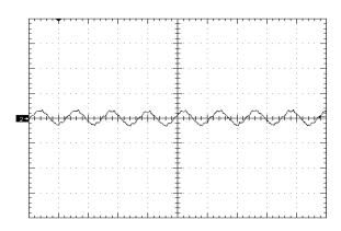
Figure 6. Input Reflected Ripple Current (20mA/div) time scale - 2uS/div. Vin=Vin\_nom, full resistive.
