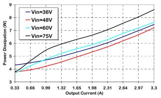
Figure 2. Power Dissipation vs. Load Current, 300lfm airflow, 25 ℃ ambient.
