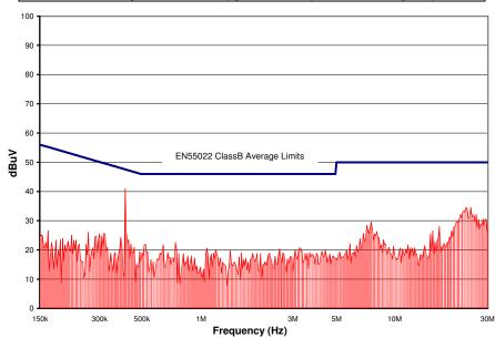
Figure 16. CPE3R48 Conducted Emissions using above specified input filter, Vin = 48V, Full Resistive Load
