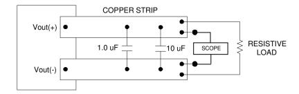
Note: Use a  $1\mu F$  X7R ceramic capacitor and a  $10\mu F$  tantalum capacitor. Scope measurement should be made using a BNC socket. Position the load 3 in. [76mm] from module.
