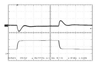
Figure 10. Load Transient Response (200mV/div), di/dt=0.1A/uS, 25% - 75% - 25% of full load +440uF output capacitance, time scale: 200uS/div
