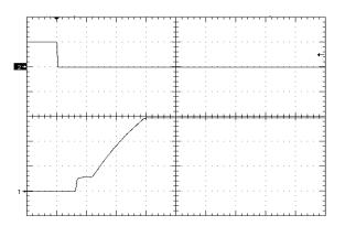
Figure 7. Startup Waveform via Enable Pin, time scale 10mS/div. Vin=Vin\_nom, full resistive load (negative enable.) Ch1=5V/div,Ch2=5V/div
