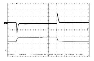
Figure 9. Load Transient Response (100mV/div), di/dt=0.1A/uS, 50% - 75% - 50% of full load, time scale: 200uS/div.
